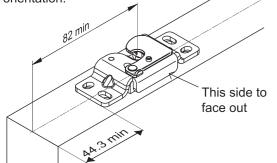
(b) Pre-drill the pilot holes for 10G screws.
