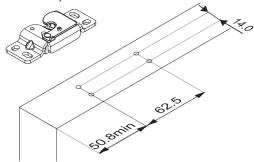
(c) Fix bracket with mounting screws provided.
